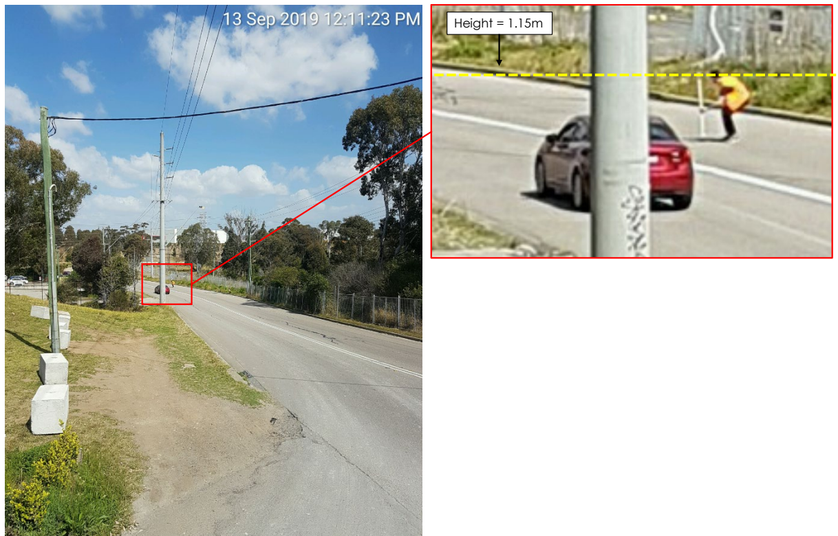
Figure 7: Sight Distance Assessment – Left-side Approach (83m at a height of 2.5m)
