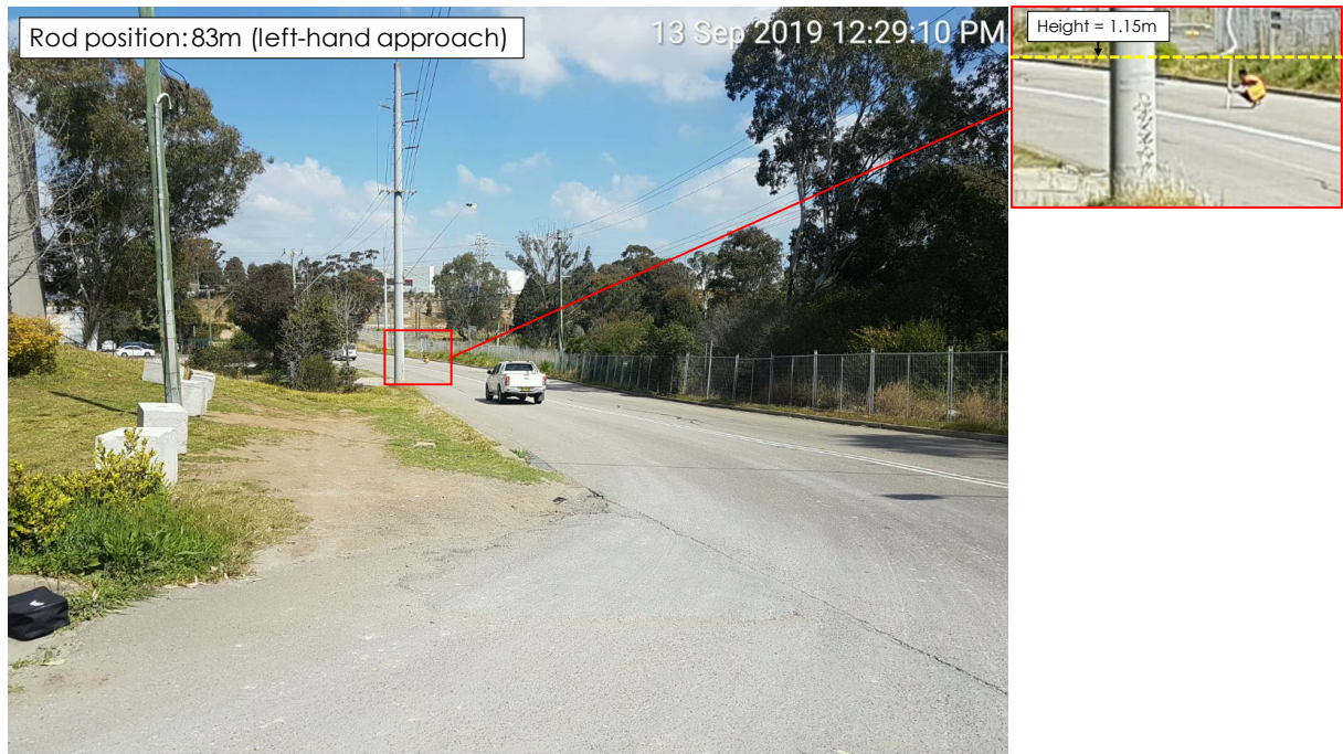
Figure 5: Sight Distance Assessment – Left-side Approach (83m at a height of 1.15m)
