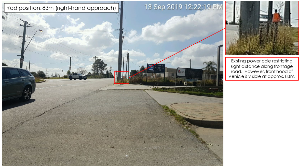
Figure 4: Sight Distance Assessment – Right-side Approach (83m at a height of 1.15m)
